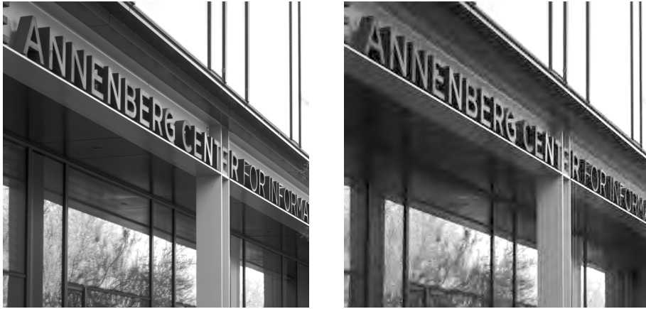
FIGURE 3.1. Images are approximately sparse in a wavelet basis. [left] A 1024 \times 1024 pixel grayscale image. [right] An approximation performed by selecting the largest 1% of the coefficients when the image is expressed in the orthonormal basis of Daubechies-4 tensor product wavelets. The reconstruction has dimension n = 1.05 \cdot 10^6 and sparsity level s = 1.05 \cdot 10^4 .
